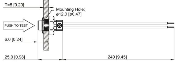
Dimension unit: mm [inch] Tolerance: +/-1 [0.04]
