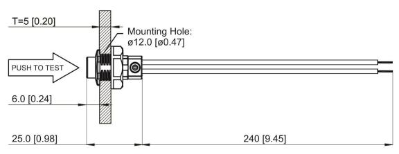
Dimension unit: mm [inch] Tolerance: +/-1 [0.04]
