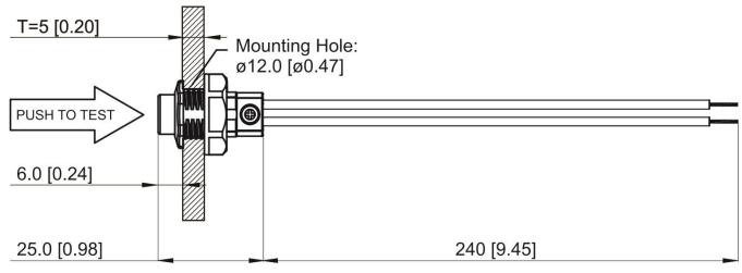
Dimension unit: mm [inch] / Tolerance: ±1 [0.04]
