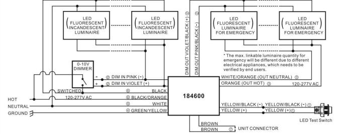
WIRING DIAGRAM FOR 0-10V DIMMABLE EMERGENCY LIGHTING SYSTEM
