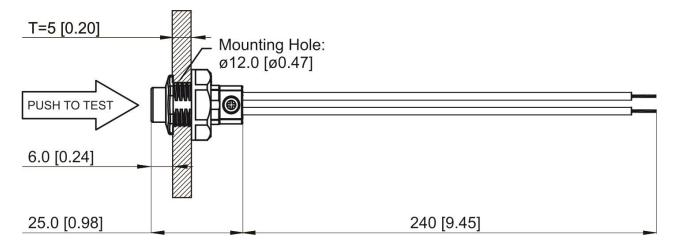
Dimension unit: mm [inch] Tolerance: ±1 [0.04]
