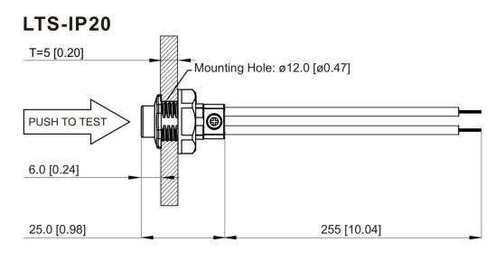
Dimension unit: mm [inch] Tolerance: ±1 [0.04]
