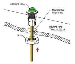
1. Test switch and LED signal lamp are in one component
