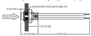
Dimension unit: mm [inch] Tolerance: ±1 [0.04]
