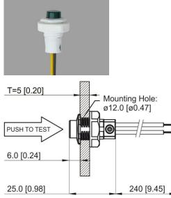
Dimension unit: mm [inch] Tolerance: +/-1 [0.04]
