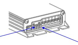
Dipswitch <u>1/2/3</u>: Setting LED working current in normal mode
