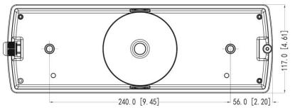
Complete lighting with1 cable gland L 358 mm x W 117mm x H 74mm Mounting distance (LF): 240mm
