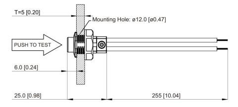
Dimension unit: mm [inch] Tolerance: ±1 [0.04]
